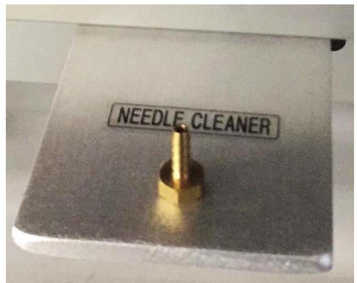
Figure 13. Needle cleaner located at base of operator panel
