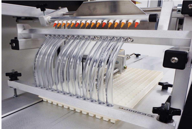
Figure 3. CE288 sowing kit attached and in place on the machine.
