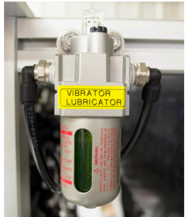
Figure 14. Vibrator lubricator on operator's right side of the machine
