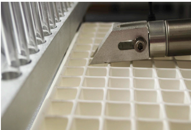
Figure 2. Tray inserted under the indexing arm and the drop tube bar.
