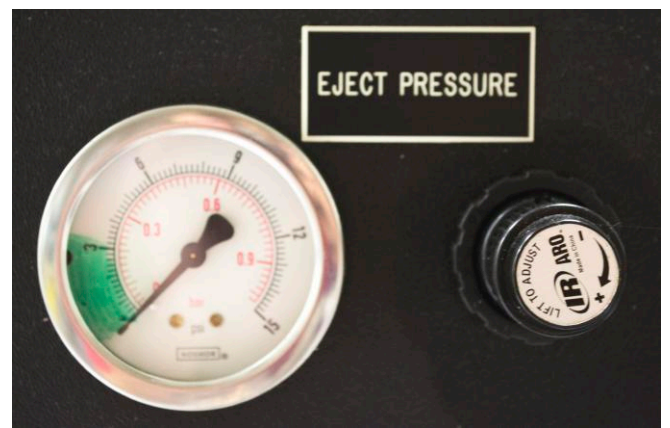
Figure 10. Eject pressure gauge and knob. Note: knob pulls out then turns right/left.
