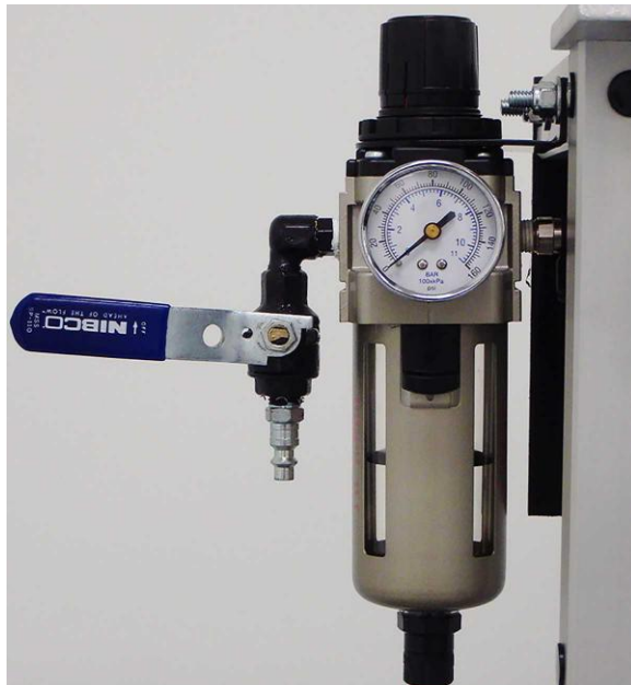
Figure 1. Filter regulator in off position. Airline connects to fitting below blue handle.
