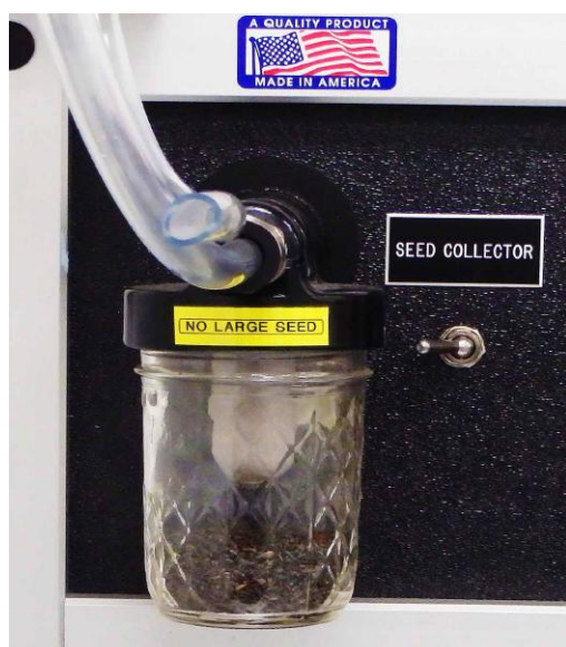
Figure 11. Seed collector & switch.
