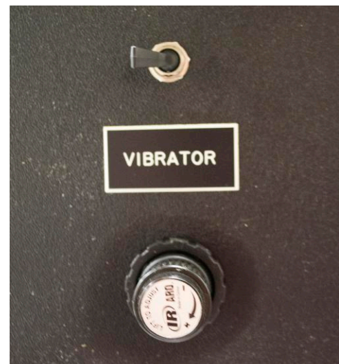
Figure 8. Vibrator switch and adjustment knob.
