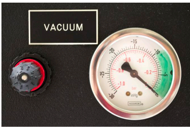
Figure 9. Vacuum knob and pressure gauge.
