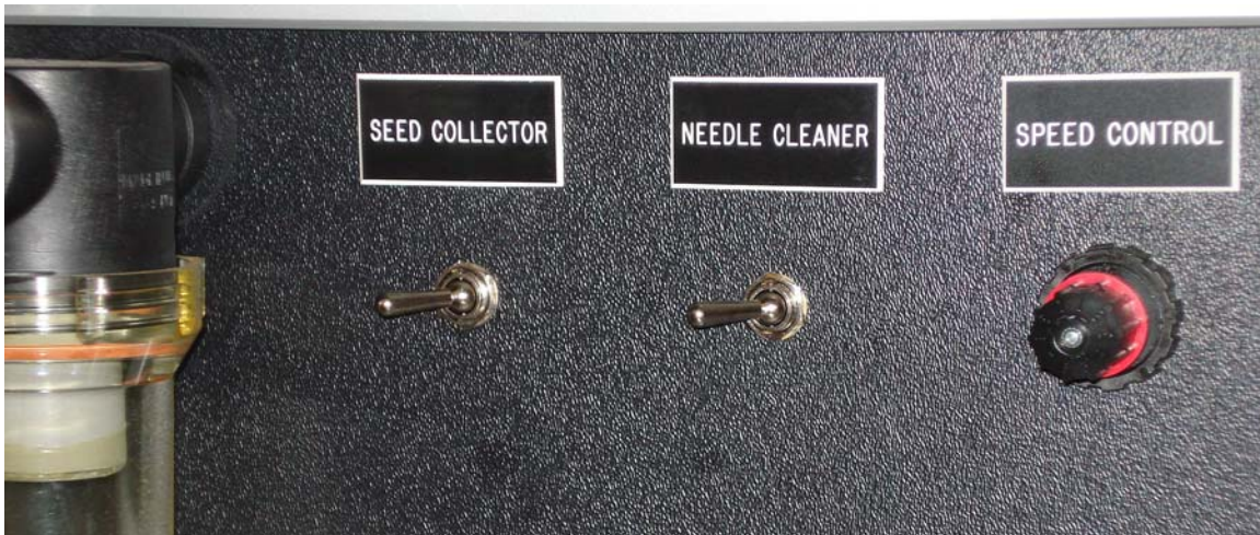
Figure 9. Seed collector, seed collector switch, needle cleaner on/off and speed control.
