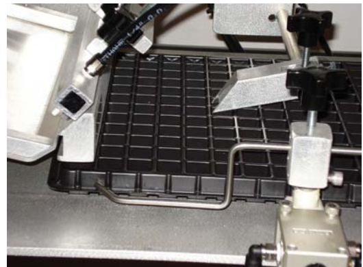
Figure 6. Tray is properly set up with first cell directly under drop tube, indexing push bar is set to forward wall of cell. In the foreground is the stainless steel vacuum actuator arm.
