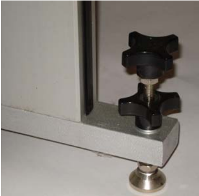
Figure 2. One of four leveling pads located at each outside corner of base of machine.
