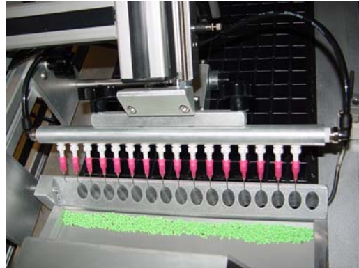
Figure 3. Seed (green) in the pan showing properly leveled machine.
