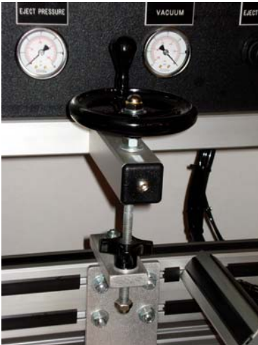
Figure 7. Height adjust arm with lower locking handle and upper adjusting handle.
