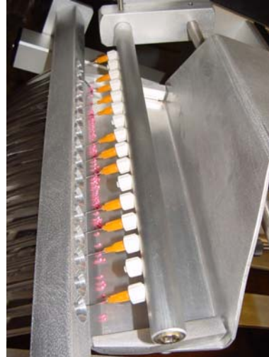
Figure 7. Seed (pink) in the pan showing properly leveled machine.
