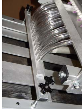
Figure 5. A TLC 200 sowing kit attached and in place on the machine.
