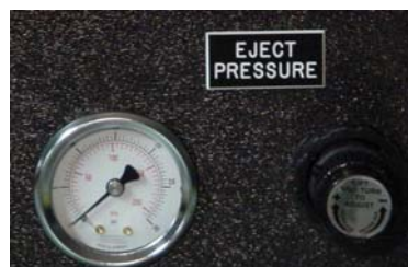
Figure 12. Eject pressure gauge and knob. Note: knob pulls out then turns right/left.
