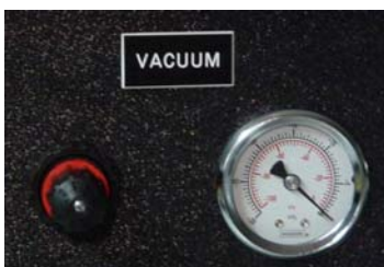
Figure 11. Vacuum knob and pressure gauge. © Seederman Seeders 2003
