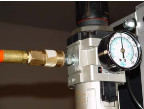
Figure 1. Regulator showing air line properly connected to valve.
