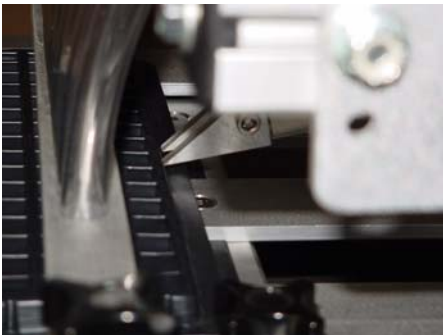
Figure 2. Tray inserted under the indexing arm and the drop tube bar.
